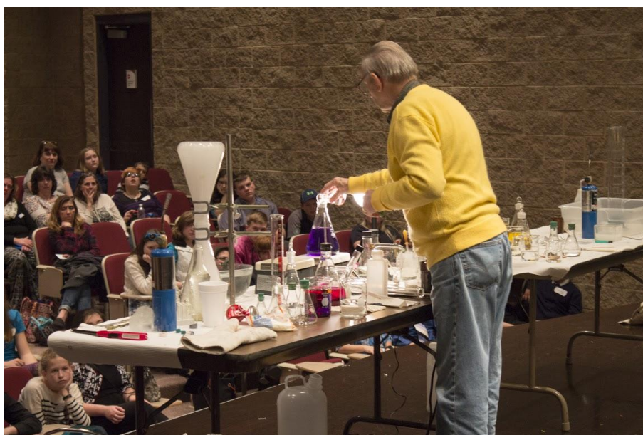
Slowly pouring a dilute solution of HCl down the side of a flask of stirred water made blue with thymolphthalein indicator and base will produce a blue tornado. The white flask turned upside down was used to illustrate the neutralization of ammonia and hydrochloric acid vapors to form an ammonium chloride cloud.
